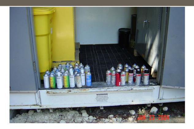
RCRA regulations require that, unless relieved of pressure, aerosol cans must be packed in a drum and manifested for hazardous waste disposal (40 CFR Part 261).
